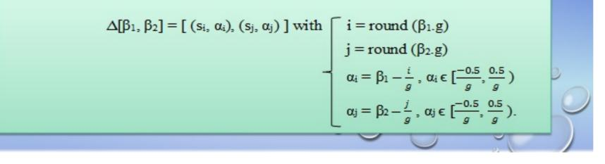
Function Δ<sup>-1</sup> converts interval 2 tuples back to interval value [β<sub>1</sub>, β<sub>2</sub>]:
